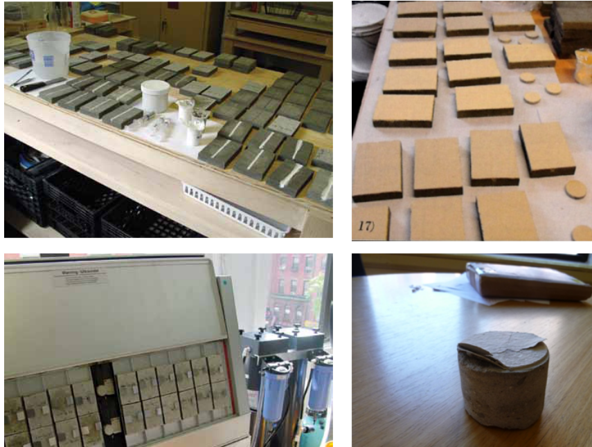
Figure 63: Samples for testing the resistance of filler products and its compatibility with the cladding. The samples are then placed in the QUV (lower right). At right, a drill core from destructive tests on the existing building. Note the number of coats of paint on the cladding
