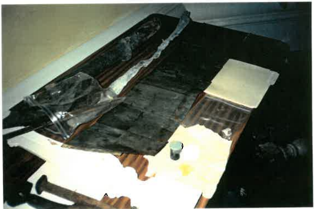
Collection of artefacts. Elements from the tinplate roofing materials from the cupola, built with a "Philibert Delorme" timber structure, known through X. Ray Studies
