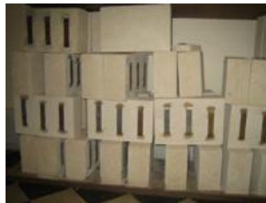
The analysis of the anchorage metals and the mortar applications in limestone.
